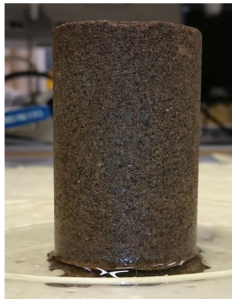
Fig. 2. Outcrop sandstone core used in the flooding experiment.
