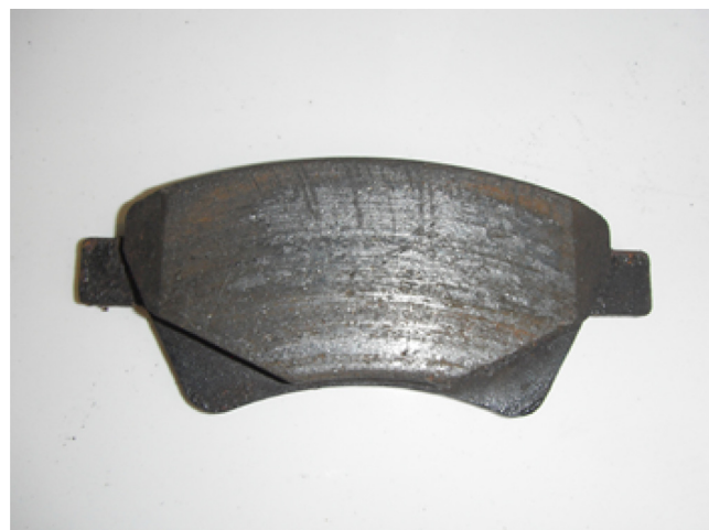
Fig. 1. Commercial brake pad after braking test.
