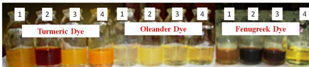
Fig. 2. Image of extracted dyes from various sources (1-aqueous, 2-alkaline, 3-alcoholic and 4-acidic).
