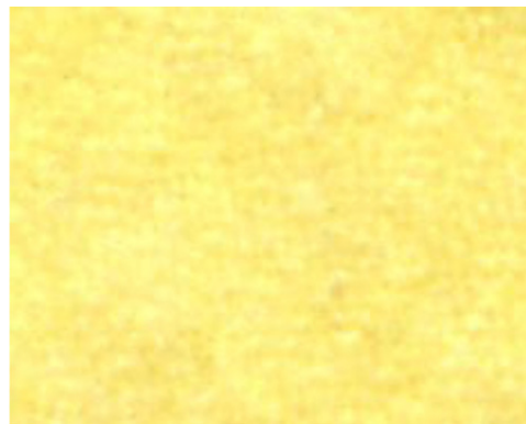
Fig. 2. Photography of dyed wool fabric. Dyeing conditions: C_{\text{indicaxanthin}} 20 mg/L, pH 4, LR 40:1, 90 min, and 70 °C.
