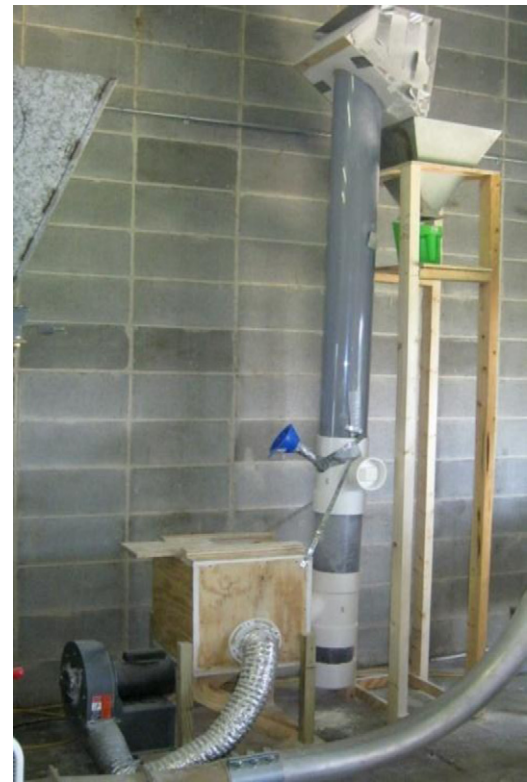
Fig. 2. Photograph of elutriation column set-up for measuring particle terminal velocities.
