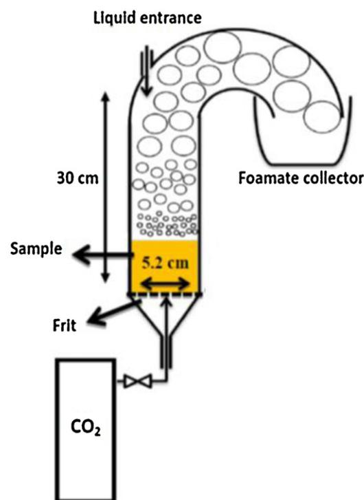
**Fig. 1.** Schematic diagram of CO<sub>2</sub> foam fractionation system.
