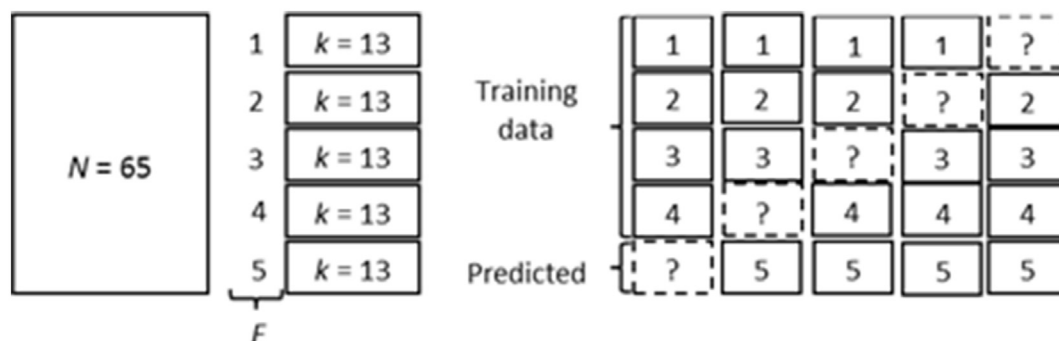
Fig. 1. Diagram of cross-validation procedure. N is the total number of data, F is the number of groups and K is the quantity of data of each group.
