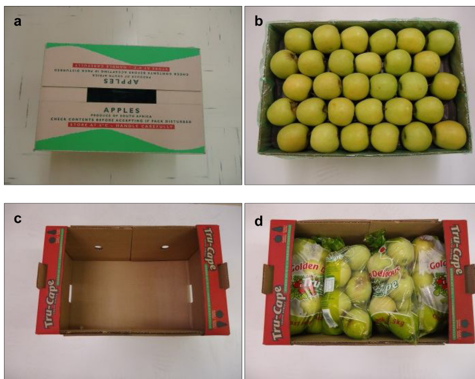
Fig. 1. Packaging designs used: (a) MK4 box; (b) tray arrangement in MK4 box; (c) Econo box; (d) fruit packed in plastic bags arranged in bulk inside Econo box.
