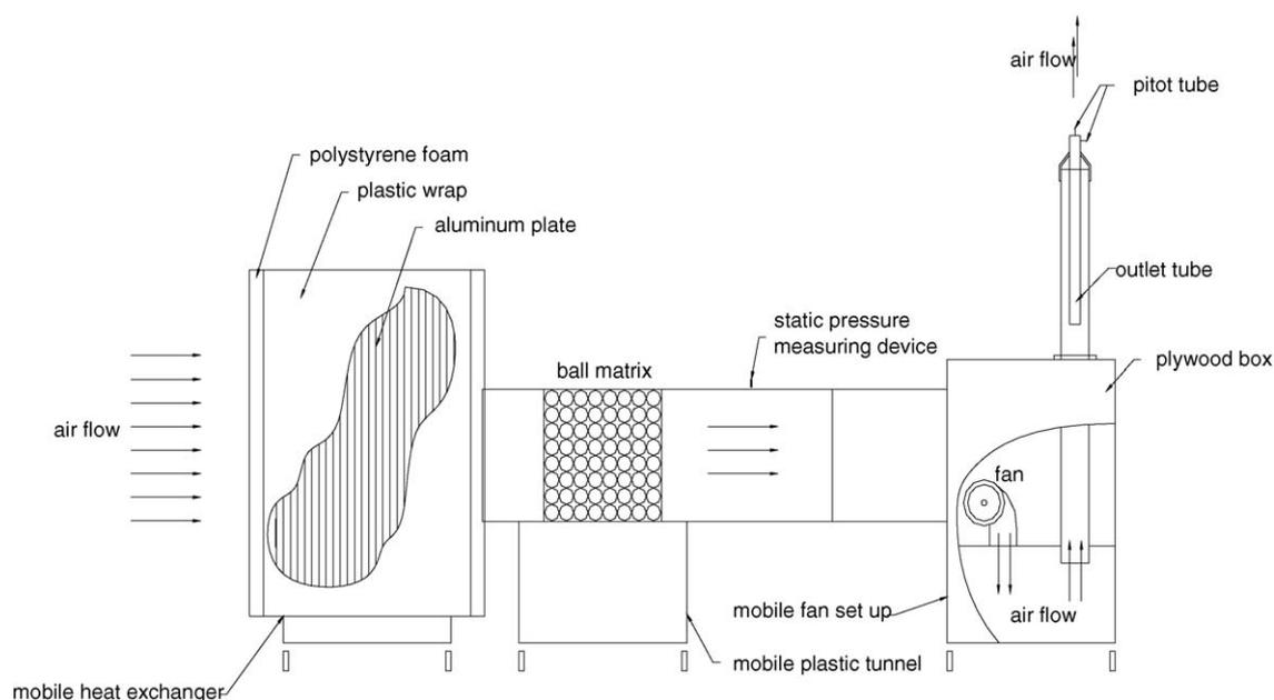
Fig. 1. Experimental set up showing forced air tunnel, balls matrix, fan, and air pressure drop and flow rate measuring devices.
