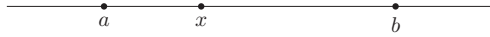
Fig. 1. The left fractional derivative of a function depends on points from a left endpoint a up to the point of evaluation x . The right fractional derivative depends on points from x up to a right endpoint b .
