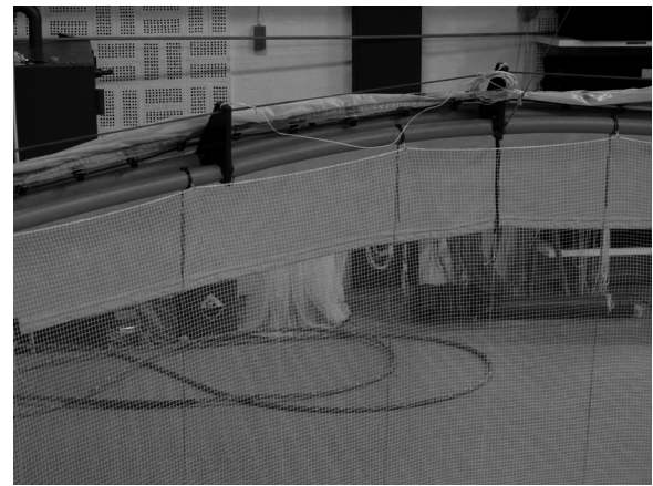
Fig. 1. Model cage with a floating collar consisting of two PE80 tubes, a nylon net with solidity 21%, and a skirt from waterproof parachute material.
