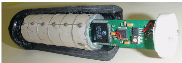
Fig. 1. Exploded view of the digital hydrophone, the coating was removed to expose the electronic board in the stack of ceramics.
