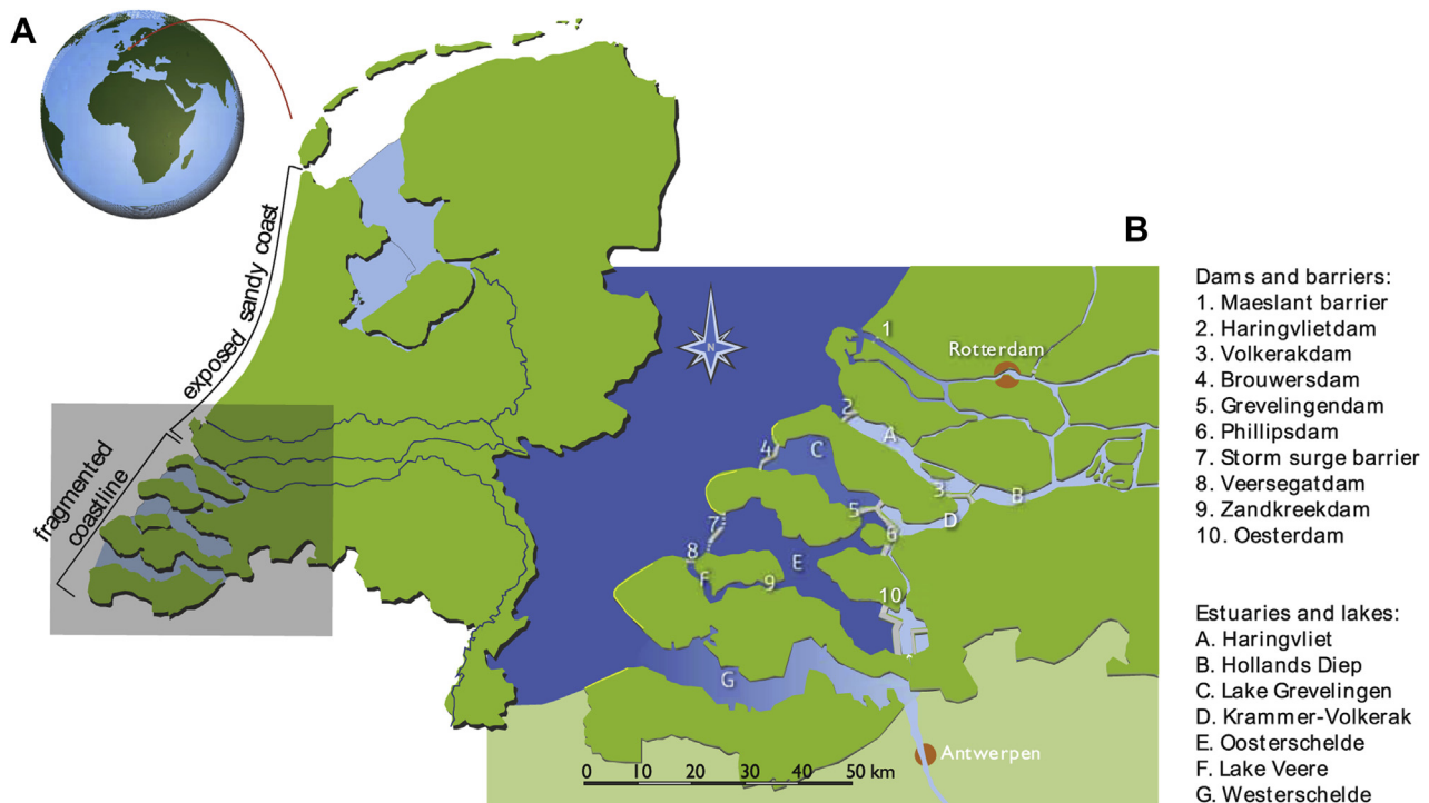
Fig. 1. Coastal management strategies in the Netherlands ( 51^{\circ} 32' 39.84'' N, 3^{\circ} 53' 11.23'' E) differ along enclosed coastlines (A) and along more complex estuarine coastlines (A and B). The Dutch Deltaworks close off the major part of the Rhine-Meuse delta, resulting in fragmented water bodies with different management problems (B). Numbers indicate dams and letters indicate water bodies. Different shades of blue indicate different salinities (light blue/light grey water is fresh and dark blue/dark grey water is salt).
