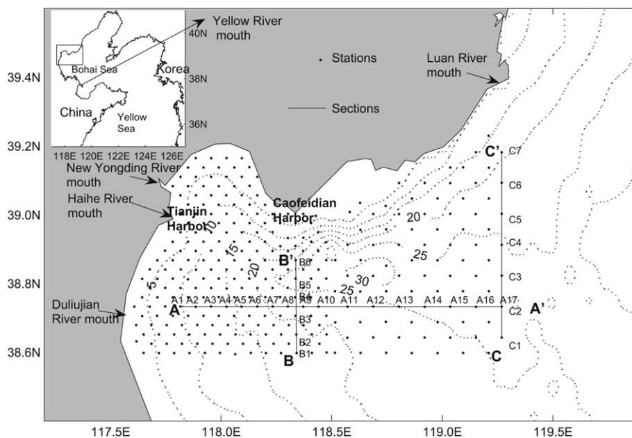
Fig. 1. Distribution of observation stations in the northern Bohai Bay. Black dots denoted stations, dashed lines indicated water depth in meter and thick lines showed sections.
