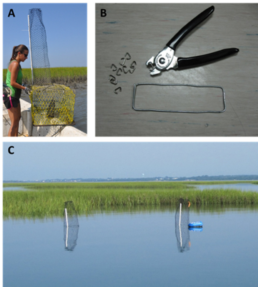
Fig. 1. Field deployments. A) Standard commercial crab pots ( 61 \text{ cm} \times 61 \text{ cm} \times 61 \text{ cm} ) were fitted with a chimney ( 122 \text{ cm} \times 30.5 \text{ cm} diameter) constructed from chicken wire to allow entrapped terrapins access to air during all phases of the tidal cycle. B) Bycatch reduction devices constructed from 12 gauge galvanized wire, hog rings, and hog ring pliers. BRDs were two different dimensions, 5.1 \text{ cm} \times 15.2 \text{ cm} (large) and 3.8 \text{ cm} \times 15.2 \text{ cm} (small). C) Modified crab pots deployed in water in the paired pot design during the 2012 field season. A pot fixed with a BRD was always placed next to a control pot (not shown).
