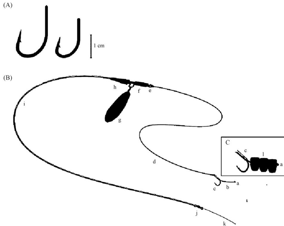
Fig. 1. Illustrations of the hook sizes used in the present study (plot A), the rig used in this study (plot B) and the hair baited with corn (plot C): (a) boilie stopper, (b) hair, (c) hook, (d) leader, (e) swivel, (f) clip, (g) lead sinker, (h) rubber, (i) braided line with a lead core, (j) swivel, (k) braided main line, and (l) corn.
