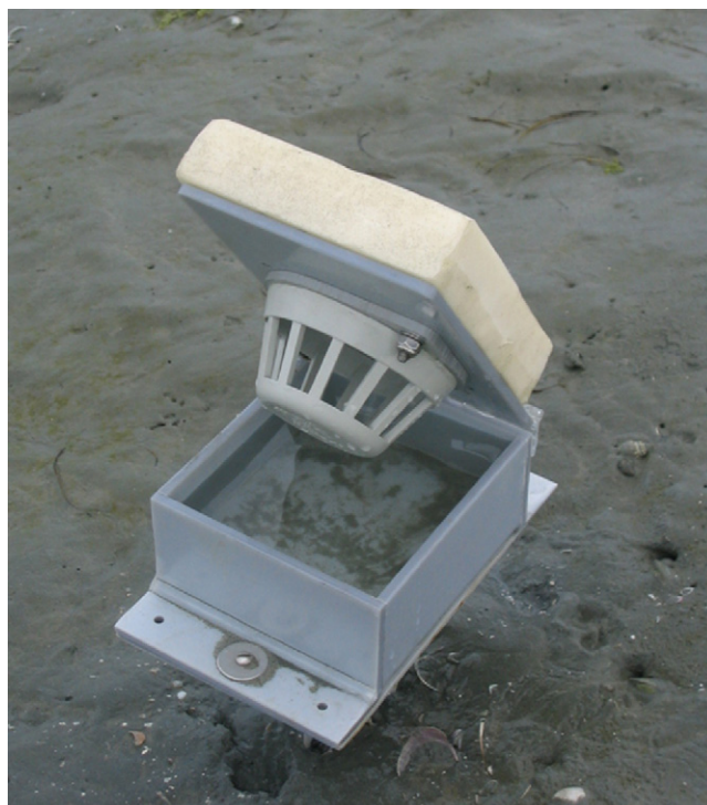
Fig. 3. “Clam” sampler with the buoyant lid held open. The SPATT bag was placed in the plastic cage under the lid of the sampler.
