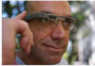
Fig. 1. Google Glass has a built in camera, microphone, speakers, touch pad, and numerous sensors [7].
