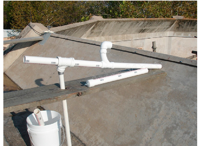
Fig. 1. Peanut butter tube suspension apparatus viewed from the side. The tube about to be put into the corral is in front of the suspension system and the fishing line is run through the larger PVC and wrapped around the top extension to secure it.
