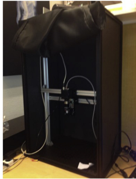
Fig. 1. Illustration of the computer vision system set-up. Camera and projector are placed in the same height. Both instruments are connected to a computer handling projections and camera trigger.
