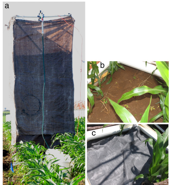
Fig. 1. Rainfall simulator and details of the plots used in the study. a) General view of the tower used to support the nozzle and the tarps to avoid raindrops deviation in the field. b) Bare soil corresponding to the high kinetic energy wetting treatment (HKE). c) Covered soil corresponding to the low kinetic energy wetting treatment (LKE).
