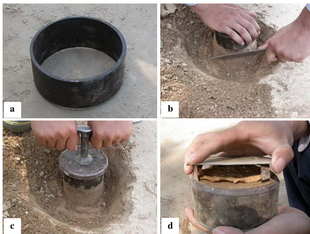
Fig. 1. The process of taking samples from road surface with an iron ring (software used: ACDSee and Microsoft Paint).
