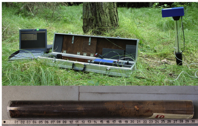
Fig. 2. Photograph of the field measurement performed with SM-400 device, and an example of soil core collected in the study area.
