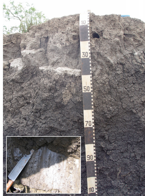
Fig. 2. A typical Vertic Planosol of the Gilgel Gibe catchment showing sub-soil gilgai and nicely developed slickensides (see inset) in the subsoil.
