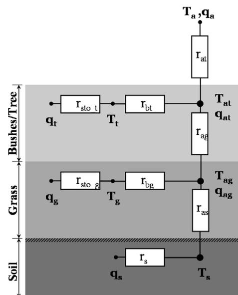
Fig. 1. Representation of the surface resistance network in the *SEtHyS\_Savannah* model: at the soil surface (mulch resistance), in the grass and bushes layers and above the vegetation (aerodynamic resistances).
