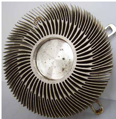
Fig. 1. Heat radiator shaped like a thick junction with the branched structure.
