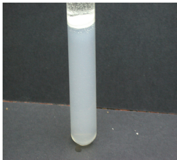
Fig. 3. Growth of SMHP crystals SD process with the sun light exposed medium at 44 °C.
