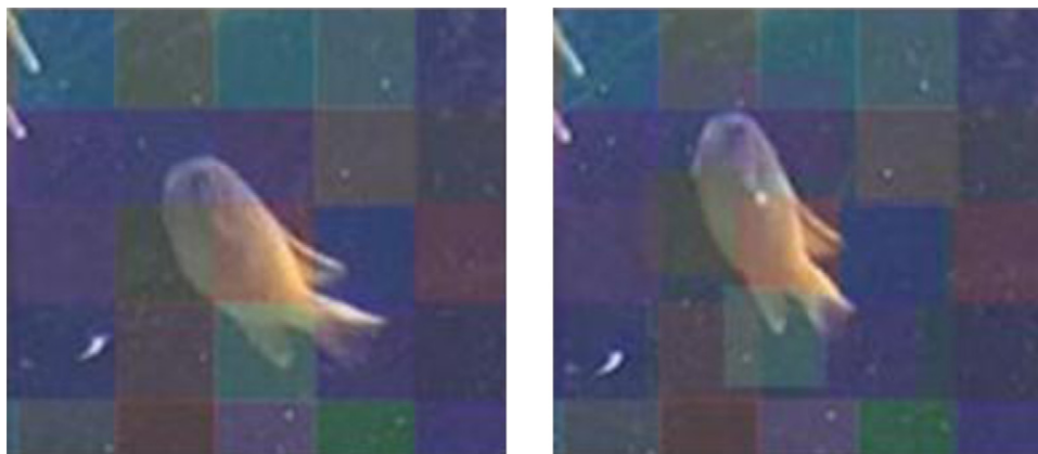
Fig. 2. Left: Block set of original image. Right: Motion estimation of blocks after scene move.
