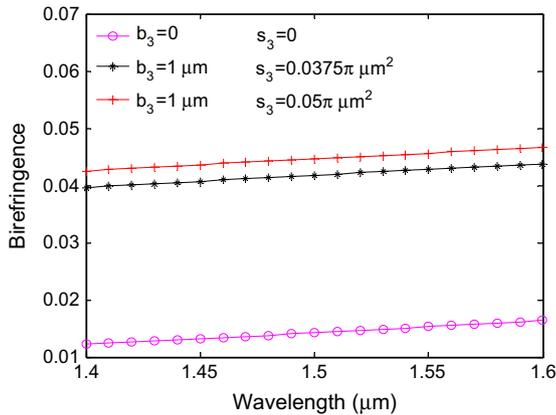
Fig. 3. The birefringence for case with  $b_3 = 1 \mu\text{m}$ .
