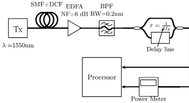
**Fig. 1.** Simulation setup: BPF – band pass filter, BW – bandwidth,  $\tau$  – time delay of the interferometer, EDFA – erbium doped fiber amplifier, SMF – single mode fiber, DCF – dispersion compensating fiber, and NF – noise figure.
