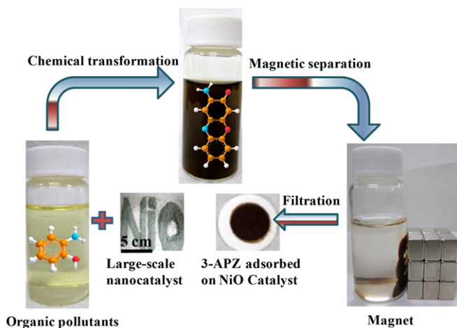
Scheme 1. Catalytic transformation and removal of organic pollutants (3-APZ) using mesoporous NiO NM.
