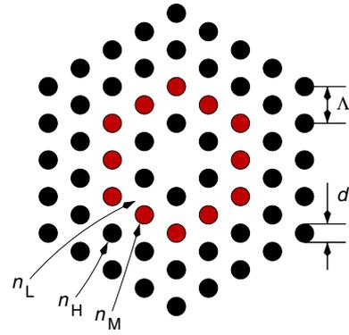
**Fig. 1.** All-silica PCF with low index silica matrix ( $n_L$ ), high index inclusions ( $n_H$ ) in the cladding and modified index inclusions ( $n_M$ ) in the second period of the photonic crystal cladding. The pitch of the fibre is  $\Lambda$  while the diameter of the inclusions are uniform with a diameter of  $d$ .
