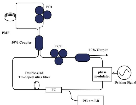
Fig. 1. The experimental setup of the proposed multiwavelength TDFL.
