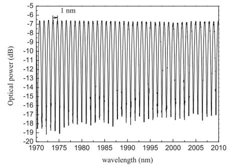
Fig. 2. The transmission spectrum of the PMF–SLM filter.
