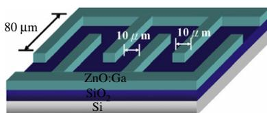
**Fig. 1.** Schematic diagram of the patterned ZnO:Ga film after the etching process.
