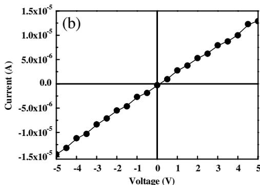
**Fig. 2.** (a) FESEM image of the ZnO nanowires grown on the ZnO:Ga/SiO<sub>2</sub>/Si template. The inset shows Enlarged SEM photographs of the ZnO nanowires grown on the SiO<sub>2</sub> spacer regions. (b) I–V characteristics measured from the two electrodes of the sample.
