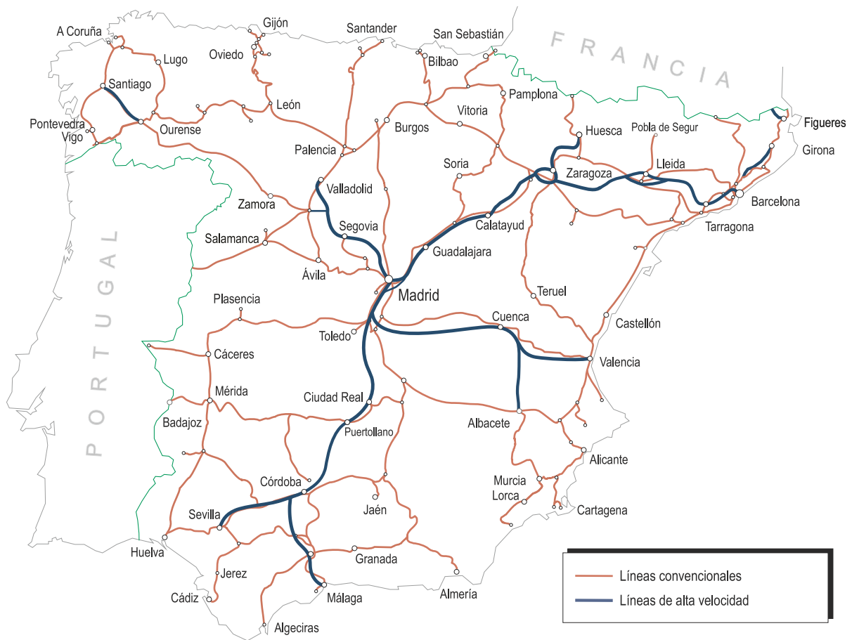
Fig. 1. Spanish railway network November 2012. The Iberian gauge conventional network is represented with thin red lines. The high speed international gauge network is represented with thick blue lines. (Courtesy of the Spanish Railway Foundation.)
