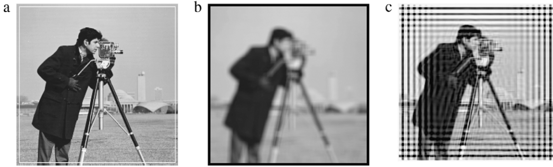
Fig. 1. An example of boundary artifacts. (a) The original image with a field of view shown in the white box. (b) Blurred image using a uniform kernel of size 9 \times 9 , where the missing boundary values are set to zeros. (c) Deblurred image with severe boundary artifacts.
