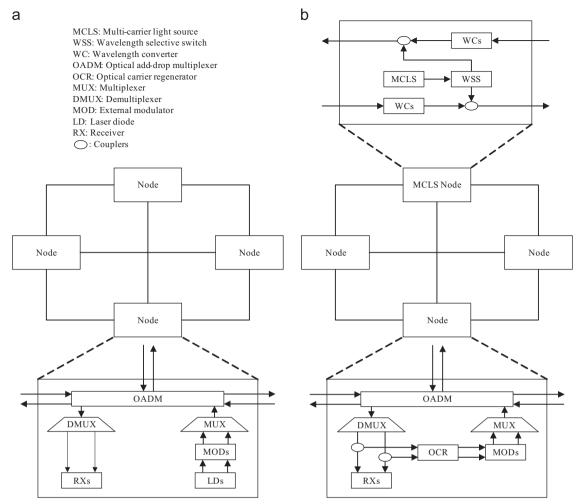
Fig. 1. Network architectures. (a) WDM network without wavelength reuse. (b) WRMD network with wavelength reuse.
