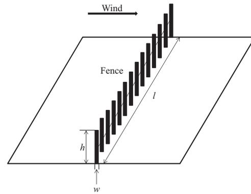
Fig. 1. Definitions of wind fence height  $h$ , length  $l$  and width  $w$ .
