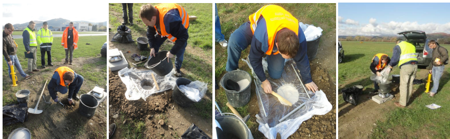
Fig. 1 A view on excavated hole and a filling with sand.
