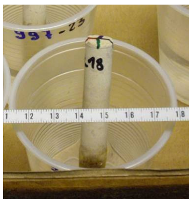
Figure 1: (a) Experiment 1 : limestone samples are drilled; drill-core is 10 cm long, and radius is 0.6 cm ; it is soaking in acidic water solution (b) Experiment 2: limestone samples are 5*5*8 cm parallelepiped with a rock bridge, of 1.5 cm of side; acidic water is added drop wise with a velocity of 1 liter per day.
