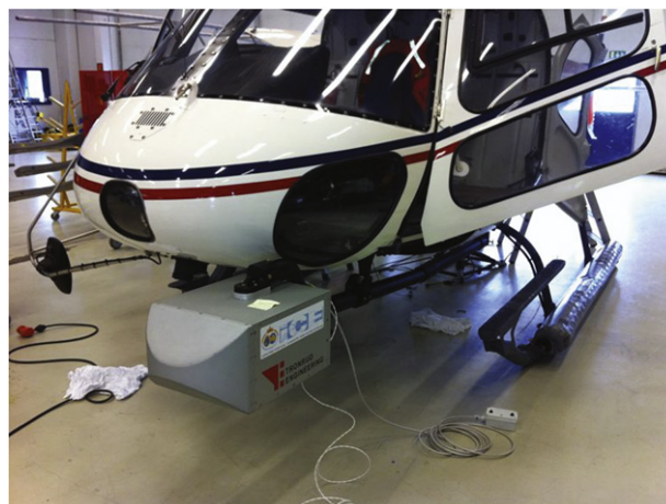
Fig. 1. Aerodynamic enclosure of ICE stereocamera system mounted on AS-350 helicopter using a single pole utility mount.
