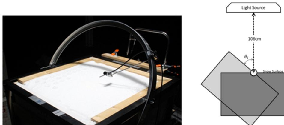
**Fig. 2.** Left: Goniometer and spectrometer configuration. Right: Sun angle  $\theta_i$  was varied by tilting the snow surface with respect to the fixed light source.
