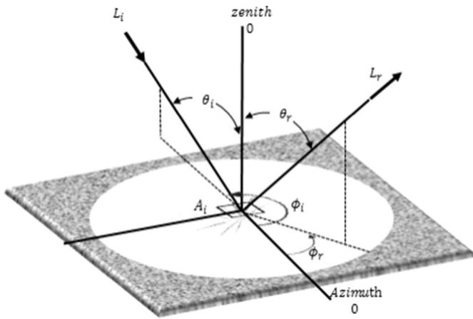
**Fig. 1.** Reflectance azimuth ( $\theta_r$ ) and zenith ( $\phi_r$ ) angle as well as incident zenith ( $\theta_i$ ) and azimuth ( $\phi_i$ ) angle. In this study, 0 azimuth is defined relative to the incident light such that  $\phi_i = 180^\circ$ .
