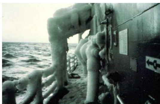
Sea spray icing on a ship. From http://upload.wikimedia.org . PART 1: PRESENTATION OF THE MODEL
