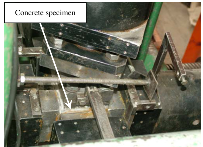
Fig. 2. The loading directions and the states of the specimen under triaxial T–C–C.
