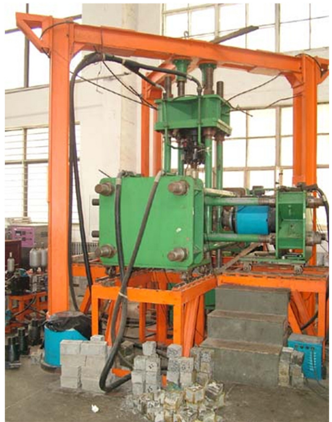
Fig. 1. The triaxial testing machine.
