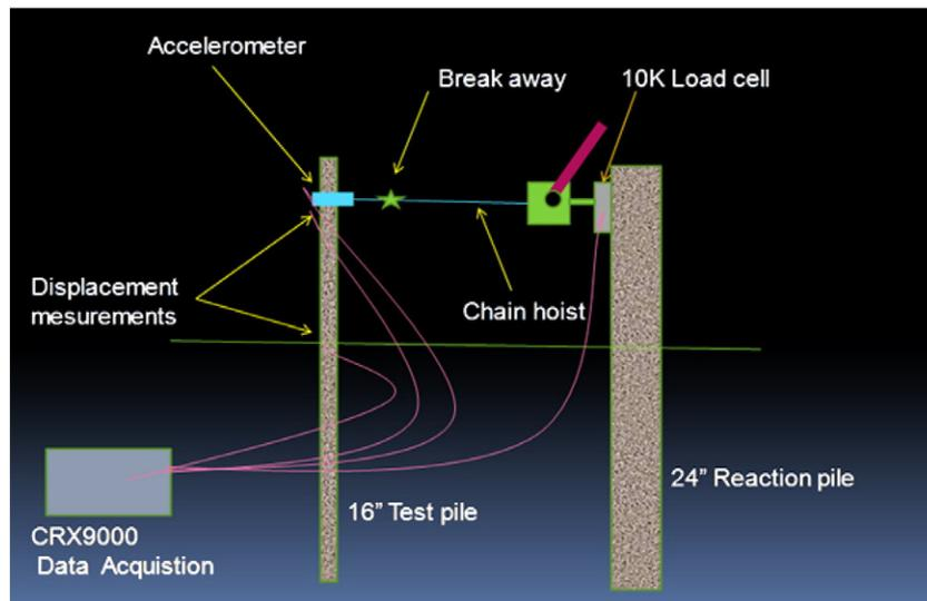
Fig. 1. Schematic diagram of the test setup.
