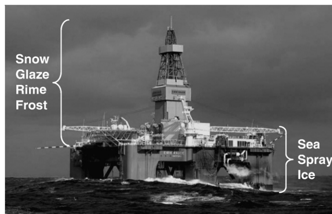
Fig. 1. Potential ice accretion areas, by ice type, on the Ocean Rig semisubmersible Erik Raude (from Paulin, 2008).
