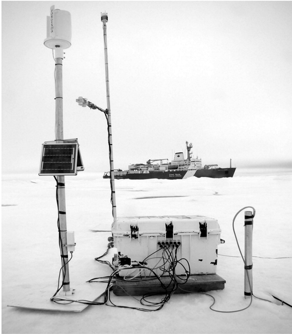
Fig. 1. A SAMS ice mass balance station in the Arctic Ocean. The solar and wind generators, together with the large battery box, could be replaced by the proposed Seebeck generator.
