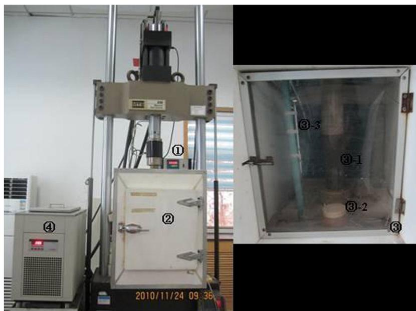
**Fig. 1.** Schematic diagram of the set up showing the sample and the machine ①-temperature controller; ②-thermostatic tank; ③-inner of thermostatic tank; ③-1-sample; ③-2-end plate; ③-3- thermistor temperature sensor; ④-cooling bath.
