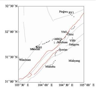
Figure 2 Locations of the leveling routes resurveyed following the Wenchuan earthquake (Gray lines represent the active faults; red lines represent the surface rupture caused by the Wenchuan earthquake)
