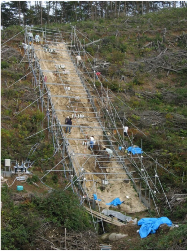
Fig. 1. Photograph of an instrumented natural hillside being prepared for a landslide-initiation experiment, Ibaraki prefecture, Japan, 2003 (see Ochiai et al., 2004, 2007). USGS photo by M.E. Reid.
