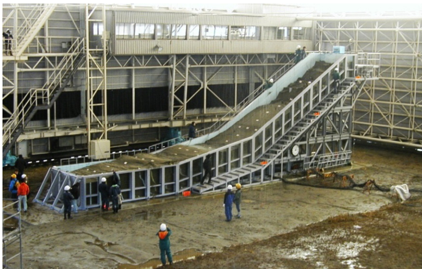
Fig. 2. Photograph of the aftermath of a large-scale laboratory landslide experiment at the National Research Institute for Earth Science and Disaster Prevention (NEID), Tsukuba, Japan, 2003 (see Moriwaki et al., 2004). NEID photo by H. Moriwaki.
